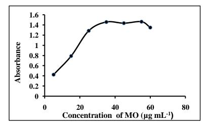
Fig.(4):- Effect of concentration of MO on the determination of SC (Conditions:  $25 \mu g SC mL^{-1}+(x) \mu g MO mL^{-1} + 5.0 mL buffer pH 3)$
