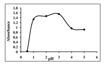
Fig. (3):- Effect of pH on the formation of the SC-MO complex (Conditions: 25 µg SC mL<sup>-1</sup> + 40 µg mL<sup>-1</sup> MO + 5.0 mL of buffer at variable pH)
