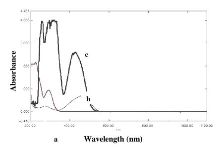
Fig. (2):- The absorption spectra of (a) SC (50 mg  $L^{-1}$ ); blank water, (b) 40 mg  $L^{-1}$  MO; blank water, and (c) SC-MO complex (25 mg  $L^{-1}$  + 40 mg  $L^{-1}$  MO + buffer solution, pH 3) in CHCl<sub>3</sub>; blank CHCl<sub>3</sub>
