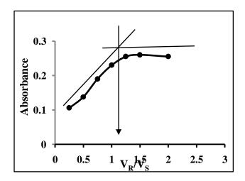
Fig .11 Mole ratio method for the compositions of SC-MO complex ( $V_R$ = volume of MO,  $V_S$ = volume of SC)
