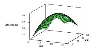
Fig (10a):- Three dimensional (3-D) RSM plot showing the effect of pH and MO concentration and their mutual effect on the absorbance
