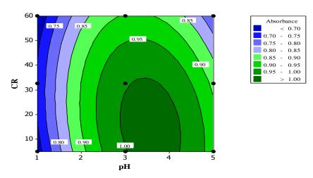
Fig (10b):- Contour plot of absorbance vs pH and MO concentration
