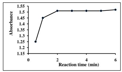
Fig.(5):- Effect of the reaction time on the formation of the SC-MO complex. (Conditions: 25 μg SC mL<sup>-1</sup> + 36 μg mL<sup>-1</sup> MO + 5.0 mL buffer pH 3)
