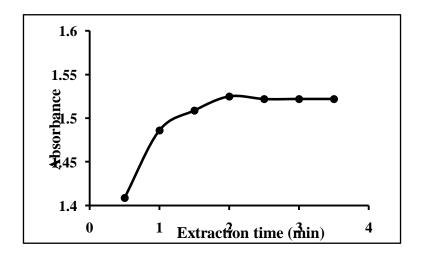
Fig. (6):- Effect of extraction time for the SC-MO complex (Conditions: 25 μg SC mL<sup>-1</sup>+ 36 μg mL<sup>-1</sup> MO + 5.0 mL buffer pH 3)
