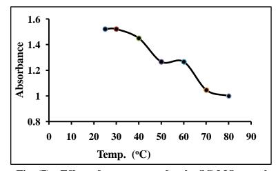
Fig. (7):- Effect of temperature for the SC-MO complex (Conditions: 25  $\mu g$  SC mL<sup>-1</sup>+36  $\mu g$  mL<sup>-1</sup> MO+ 5.0 mL buffer pH 3)
