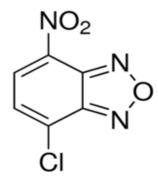
Fig. (2):- Chemical Structure of (NBD-Cl) reagent
