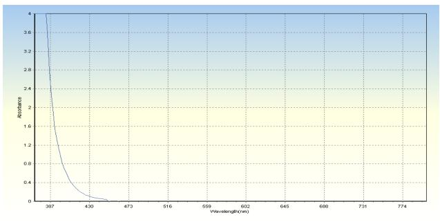
Fig.(4):- Absorption spectrum of reagent blank against ethanol
